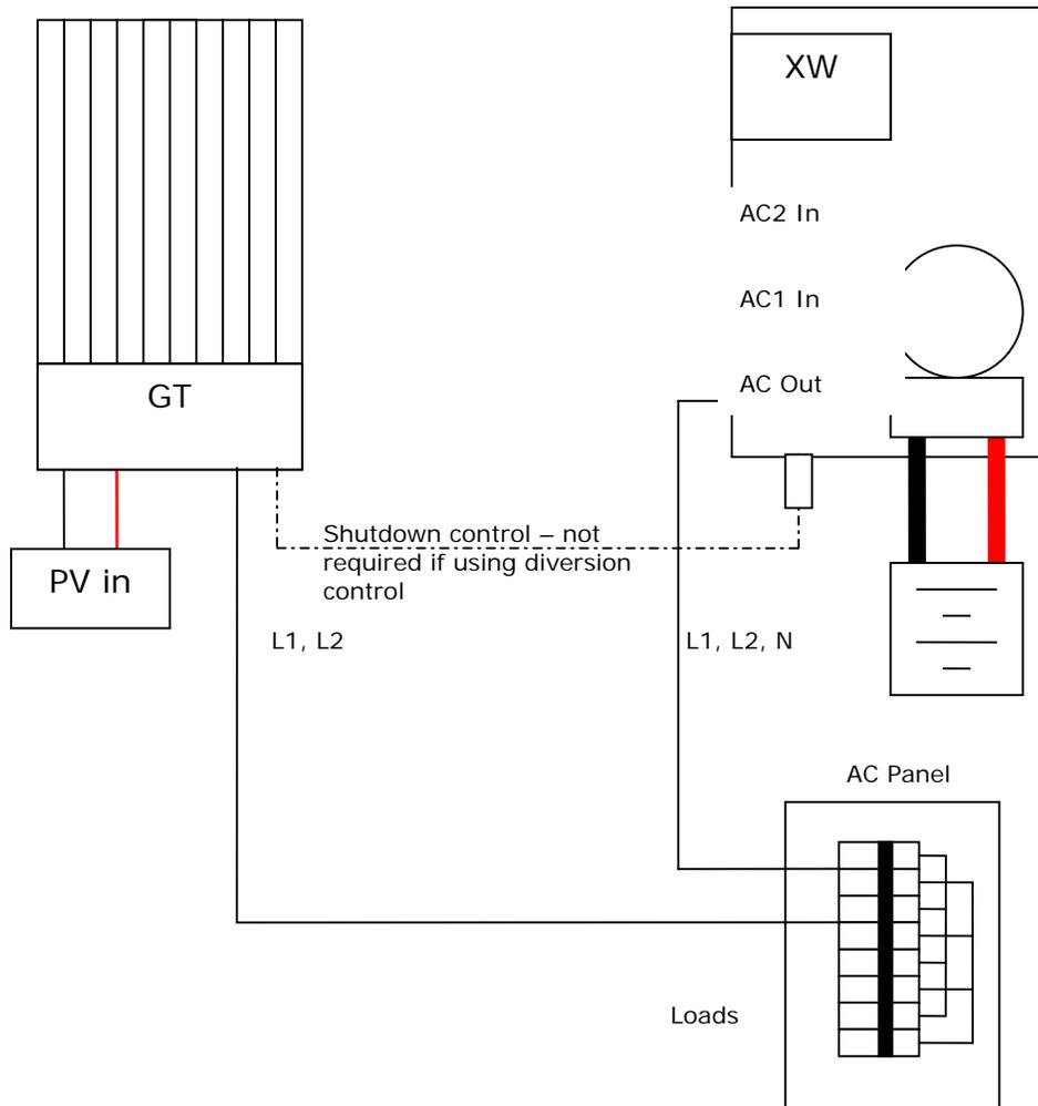
**Figure 2: AC coupled system with simple communication**
