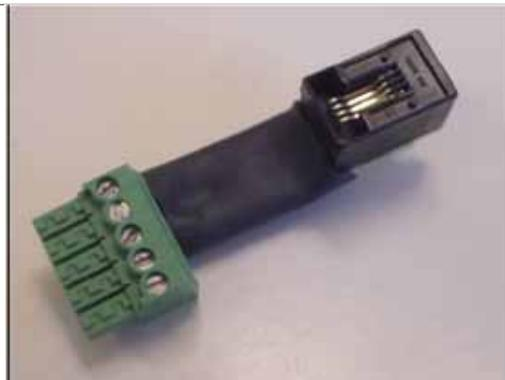
This simple communication interface enables the XW inverter to signal the GT to shutdown before the XW shuts down on "High Batt Cut Out". The AC loads will continue to operate from power produced by the XW inverter and once the battery voltage has dropped to a safe level, the XW will clear the Aux Output line which will turn the GT back on.
